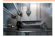
Water Resistance Highest IP-Protection Class IP69K
